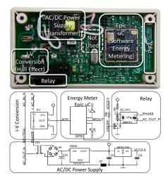
(c) ACme-B uses an in-line Hall Effect sensor as I-V conversion, a step-down transformer followed by a bridge rectifier as the AC/DC power supply, and performs energy calculation in software using the microcontroller.
