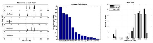
(d) Power draw of the microwaves on (e) Energy usage by plug-load type (f) Data yield from 49 nodes over a the 3rd (bottom figure) to 7th (top on a Monday averaged across all three day period. figure) floors on a typical day. loads of the particular type.
