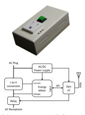
(a) ACme consists of five primary components: current-to-voltage conversion, energy metering, AC/DC power supply, microcontroller and radio, and solid state relay.
