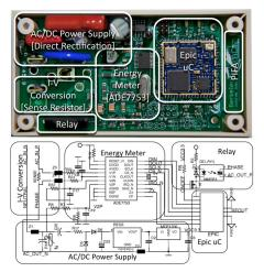
(b) ACme-A uses shunt resistor as I-V conversion, direct rectification as AC/DC power supply, and ADE7753 as the energy metering IC.
