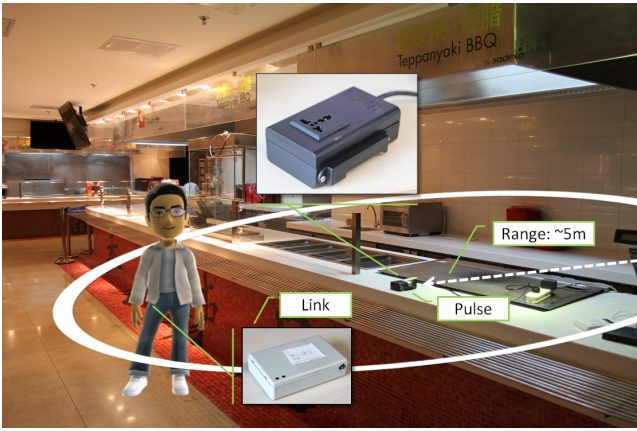
Figure 8: A Pulse is installed at the Teppanyaki counter, projecting a proximity zone of 5m radius. Links carried by diners in their pockets detect this zone as they enter.
