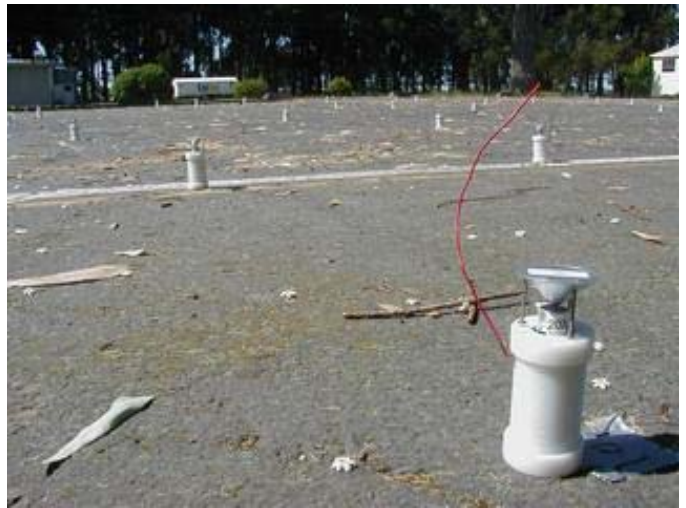
Fig. 1. Ultrasound Deployment. 49 nodes deployed in a random grid pattern in a parking lot were localized using ultrasound. The ultrasonic transducer and reflective cone are visible above the node.
